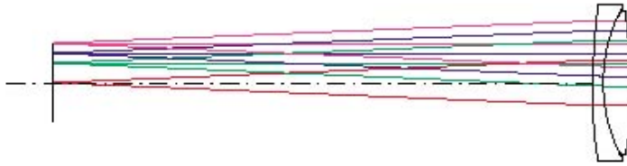
Figure A Telecentric lens drawing showing discrete object points being imaged.
